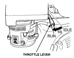
Figure 7. Throttle Lever (1/3 Start Position)
